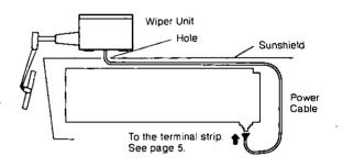
3. Attach the wiper with four screws, lockwashers and plain washers (provided with the wiper unit).
