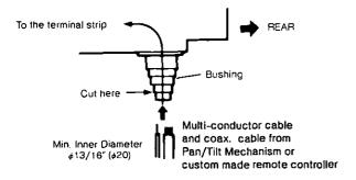
Pass the cables through the wiring hole.
