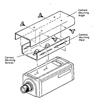
6. Adjust the camera position as shown in the drawing. Then, tighten the two butterfly screws.
