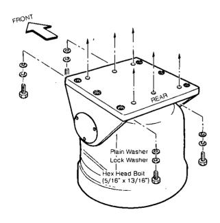
Be sure to align the camera direction and front direction of Pan/Tilt Mechanism.
