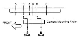
5. Attach the camera mounting plate with camera to the camera mounting angle.
