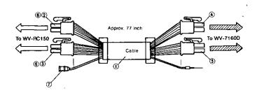
• If 13 wires cabel are avairable for WV-7160D, connect the remainded 3 wires to the ( ) position.
