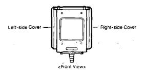
Open the right-side cover with the key (provided). If it is necessary to mount the camera from the left-side, open the left-side cover.
