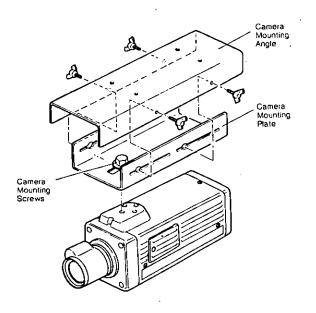
3. If it is necessary to mount the camera from the left-side, change the butterfly screws on the camera mounting angle as shown below.
